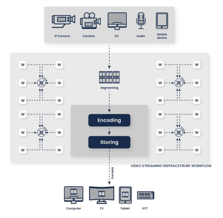
Figure. Overall workflow of AIOZ CDN
