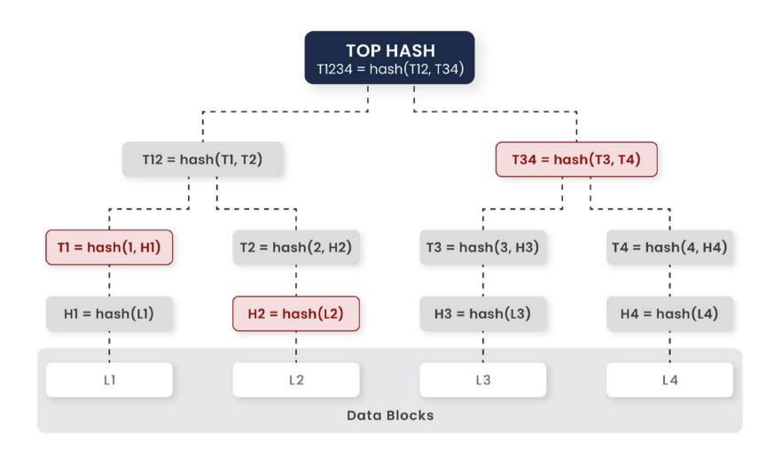
In the AIOZ Network dCDN, a complete Merkle root tree of a video segment which is being stored in Edge Nodes could be constructed from different hashes, with one hash per level being sufficient (Figure). From this tree, the HUB Node will get the final TOP HASH, whose size is log2(X) (X is the number of nodes in the tree).
