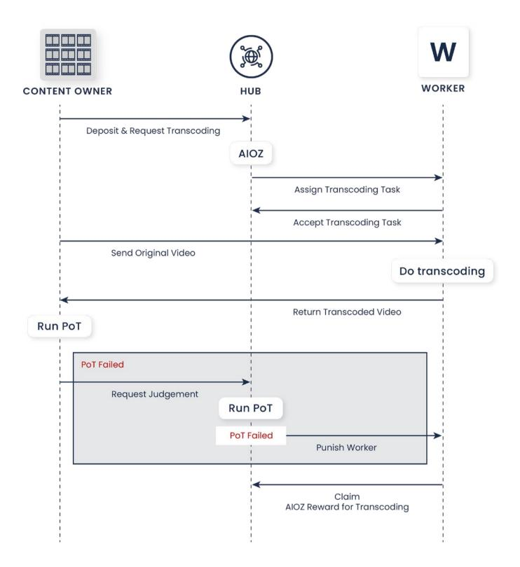
This section will elaborate on how Edge Nodes receive the transcoding task and how to prevent them from cheating (Figure). To start with, COs who want to have their videos transcoded will send their request and payment to HUB Nodes of AIOZ Network dCDN. Next, the HUB Node assesses which Edge Nodes can handle the COs' request and assigns the task to them. Edge Nodes have the right to accept or refuse the task assigned by the HUB Node as well as to freely choose which video segments to handle.
