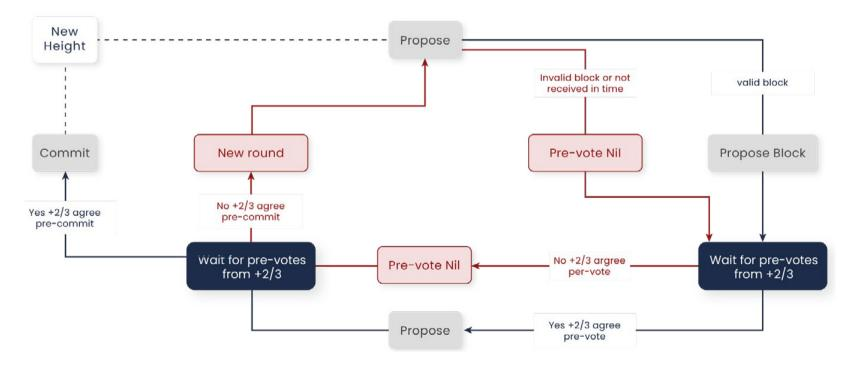
The block-proposing process is summarized in Figure: Validators take turns proposing blocks for the transaction and voting on the proposed blocks. The blocks are submitted to the chain with each block on the chain at each height. However, the block may fail to submit. In this case, the protocol will select the next certifier to propose a new block at the same height and start voting again.
