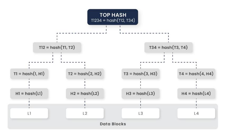
The illustration for a typical Merkle root in the AIOZ Network dCDN is shown in Figure. Instead of only 4 blocks shown in Figure, in reality, a video segment contains n blocks, in which n is computed so that the size of each block ranges from 32 to 64 bits. Via gradual pairing, we will finally achieve a TOP HASH, which is unique for one video segment. In other words, any changes in any blocks or any block disorders of a video segment will lead to a totally different TOP HASH.
