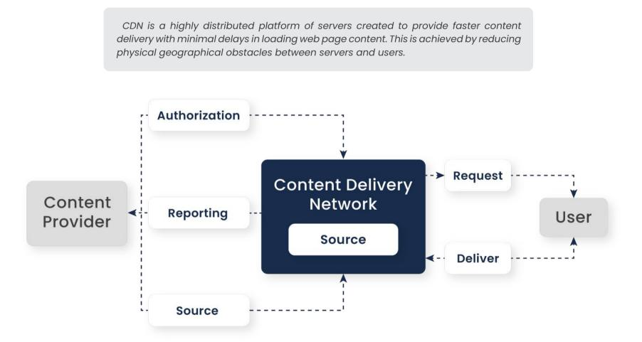
Figure. Model of a typical CDN
